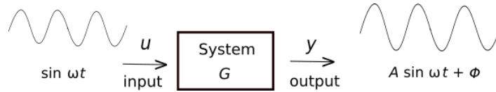
Figure 2. Sine wave in; modified sine wave out.
